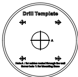
Figure 2-15 Drill Template of the Junction Box
