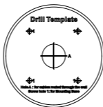
Figure 2-12 Drill Template of the Junction Box
