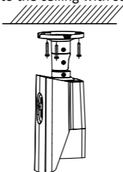
Figure 2-2 Fix the Camera to the Ceiling
