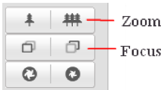
Figure 3-103 Zoom and Focus Adjustment of Electronic Lens
