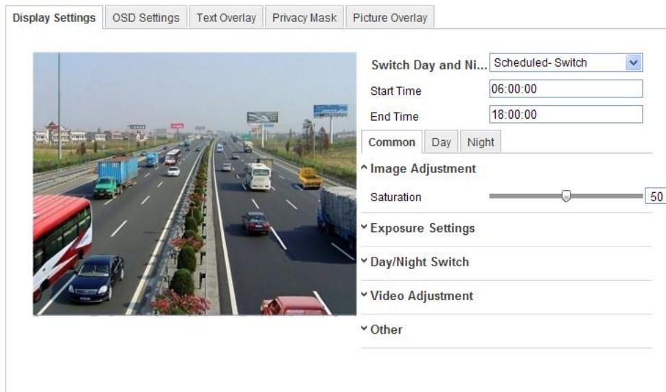
Figure 6-28 Day/Night Scheduled-Switch Configuration Interface
