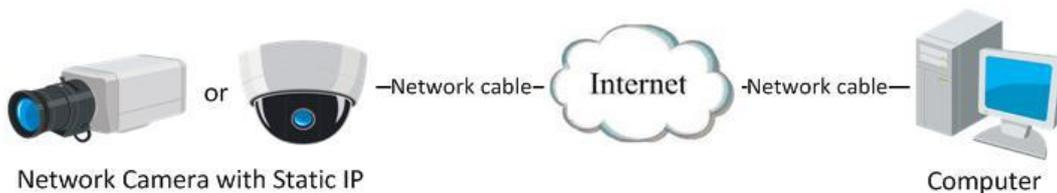
Figure 2-11 Accessing the Camera with Static IP Directly
