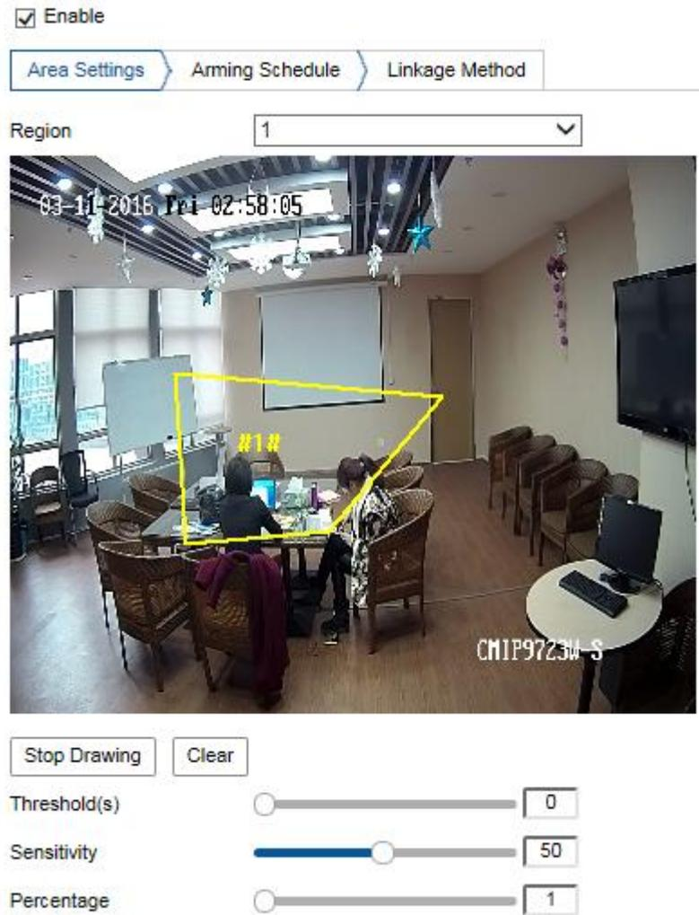
Figure 10-11 Intrusion Detection
