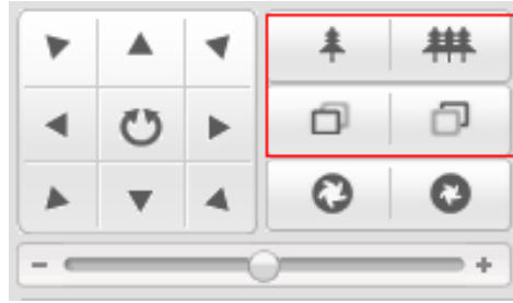
Figure 3-162 Zoom/Focus Adjustment Via PTZ Interface
