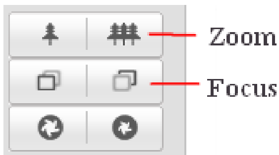
Figure 3-103 Zoom and Focus Adjustment of Electronic Lens
