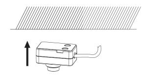
Please note that the lens direction should be in accordance with the direction of traffic.
