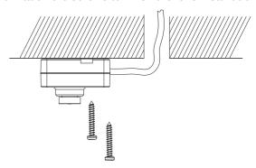
Please note that it is important to keep the lens clean when drilling holes or inserting the screws.
