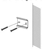
2. Hang the hook which is on upper-side of the main unit onto the rail, press a little harder on the lower part of the main unit, and then the elastic clasp will be automatically buckled.
