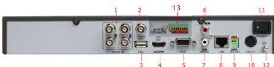
Figure 1.6 Rear Panel of 7204-WH
