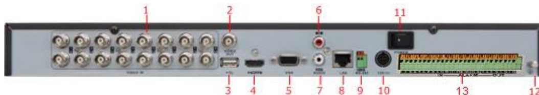
Figure 1.11 Rear Panel of 7216-WH
