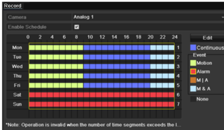
Figure 5-12 Draw the Recording Schedule
