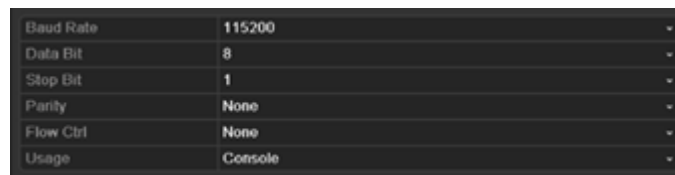
Figure 17-2 RS-232 Settings Interface
