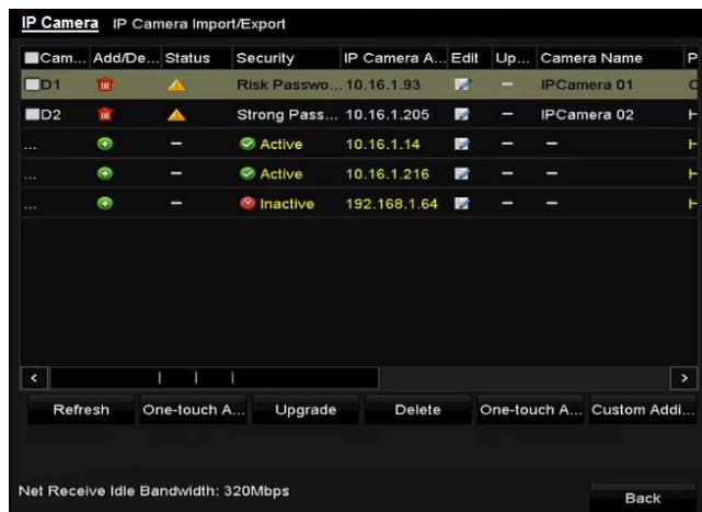
Figure 2-35 IP Camera Management Interface
