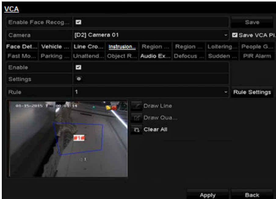
Figure 10-5 Draw Area for Intrusion Detection
