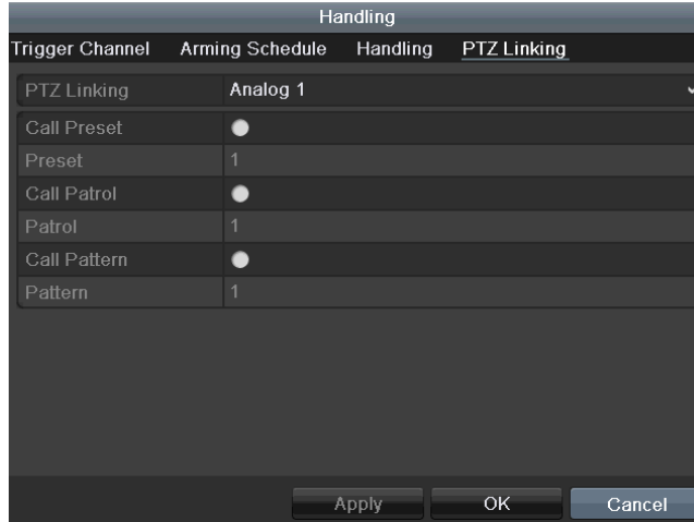
Figure 8-7 Set PTZ Linking of Alarm Input
