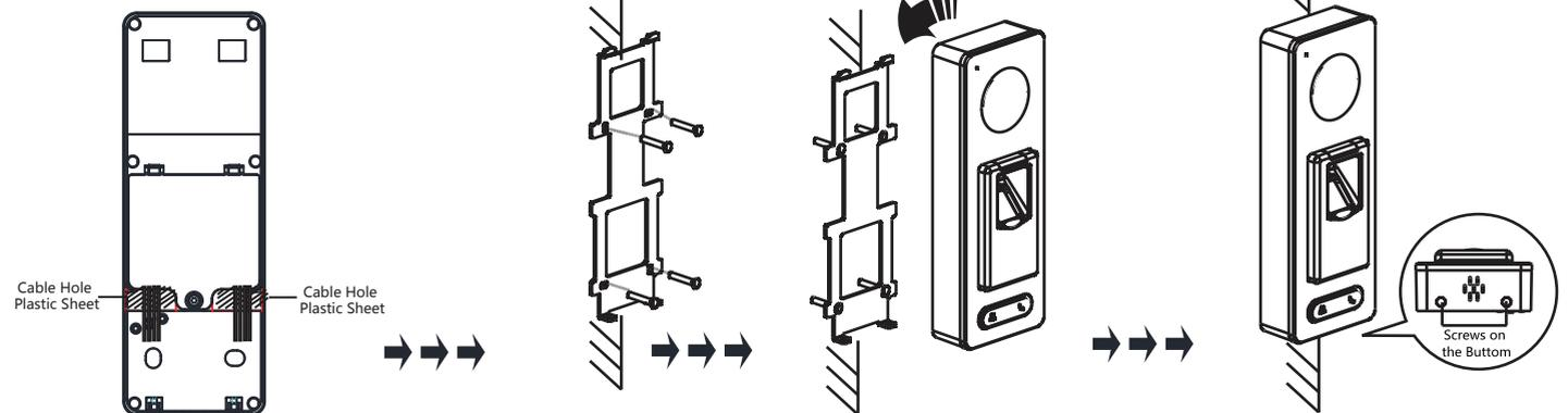
1. Connect the cables with the connector on the rear panel of the device.
