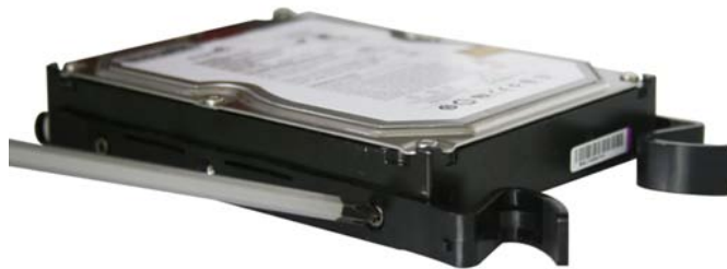
Figure 2. 1 Fasten Hard Disk
