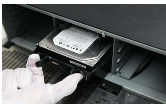
Figure 2. 4 Insert Hard Disk
