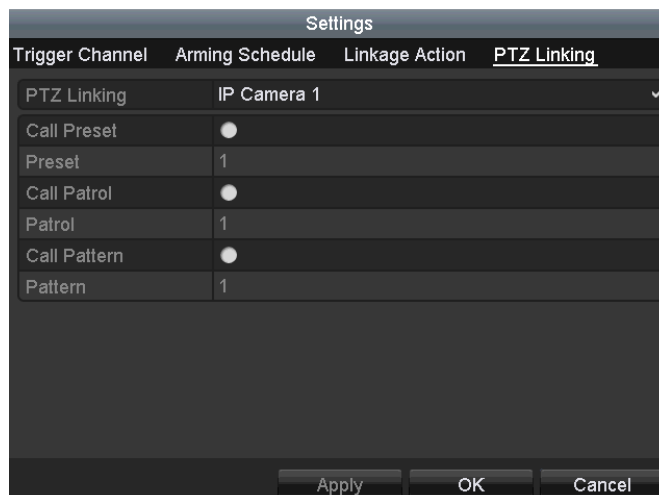
Figure 8. 6 Set PTZ Linking of Alarm Input
