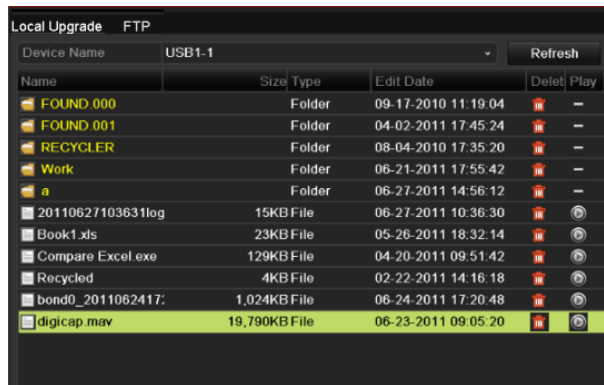
Figure 13. 7 Local Upgrade Interface
