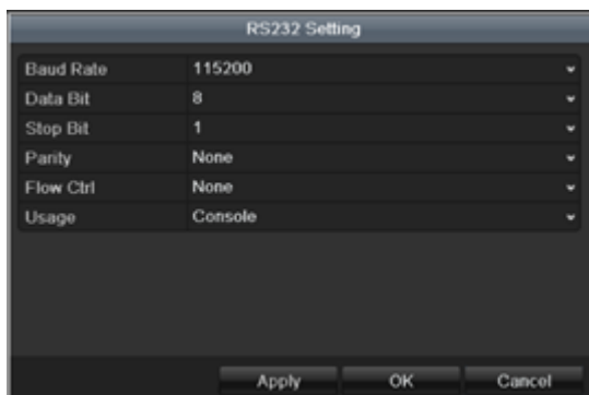
Figure 13.16 RS232-Receive port Settings Interface
