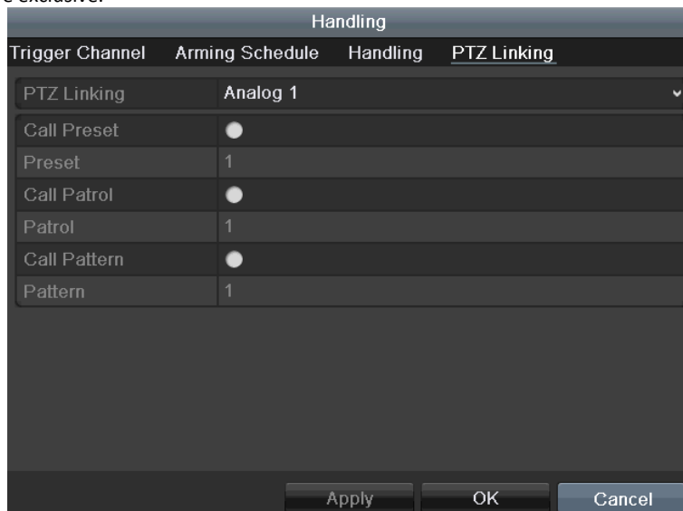
Figure 8. 8 Set PTZ Linking of Alarm Input
