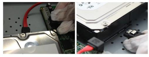
**4.** Connect the power cable to the HDD.
