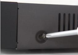
2. Install the HDD in the HDD rack using the provided screws. Fasten the screws on the bottom to fix the HDD.
