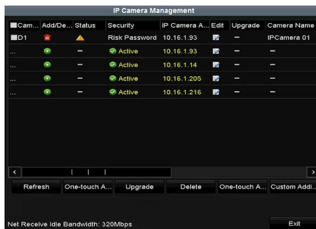
Figure 2. 19 Manual Adding IP Camera Interface
