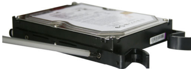
Figure 2. 1 Fasten Hard Disk
