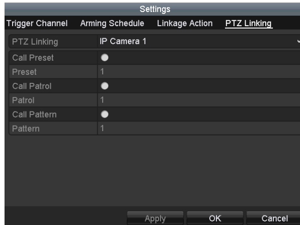
Figure 8. 6 Set PTZ Linking of Alarm Input
