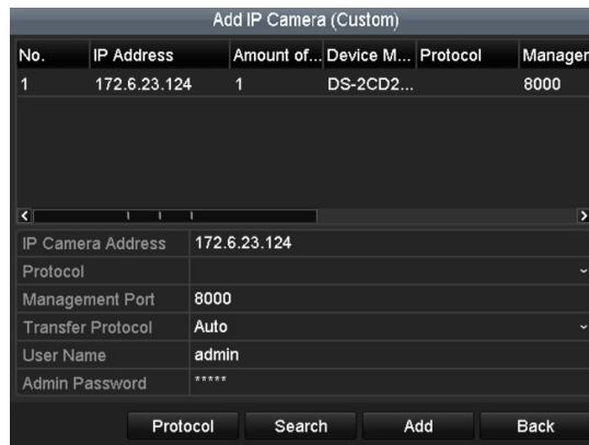
Figure 2. 23 Custom Adding IP Camera Interface
