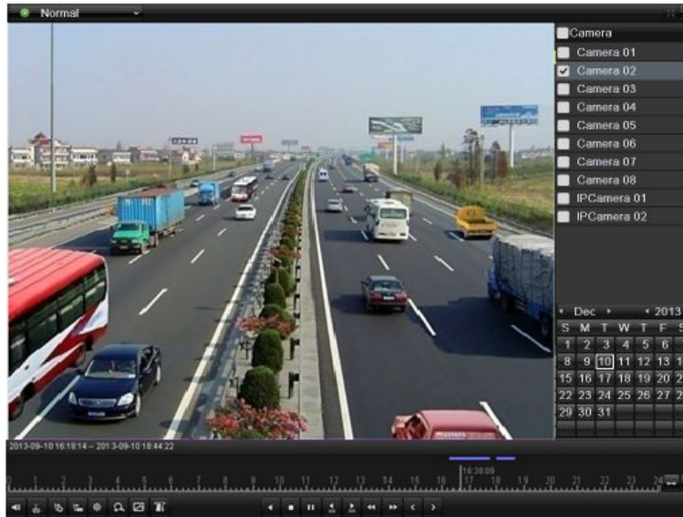
Figure 6. 12 Interface of Playback by Time
