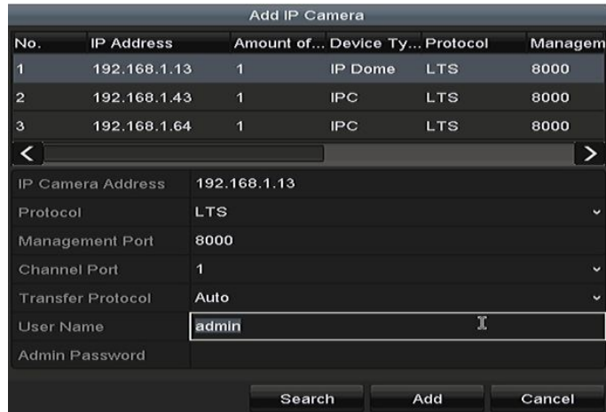
Figure 2. 20 Quick Adding IP Camera Interface
