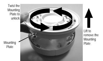
Identify components. Examine the GEMC-WL-CO to identify the component locations. Take note of the "Tamper Lock" tab located on the inside of the Mounting Plate (see image below). Optionally, cut this "Tamper Lock" tab to prevent the removal of the GEMC-WL-CO from the Mounting Plate without using a tool (such as a screwdriver).
