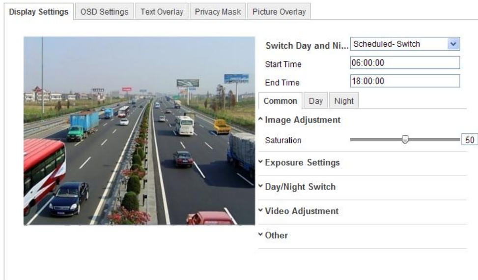
Figure 6-28 Day/Night Scheduled-Switch Configuration Interface
