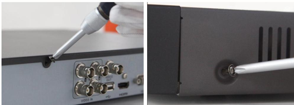
2. Install the HDD in the HDD rack using the provided screws. Fasten the screws on the bottom to fix the HDD.
