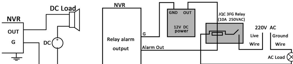
Figure 2. 7 Alarm Output Wiring
