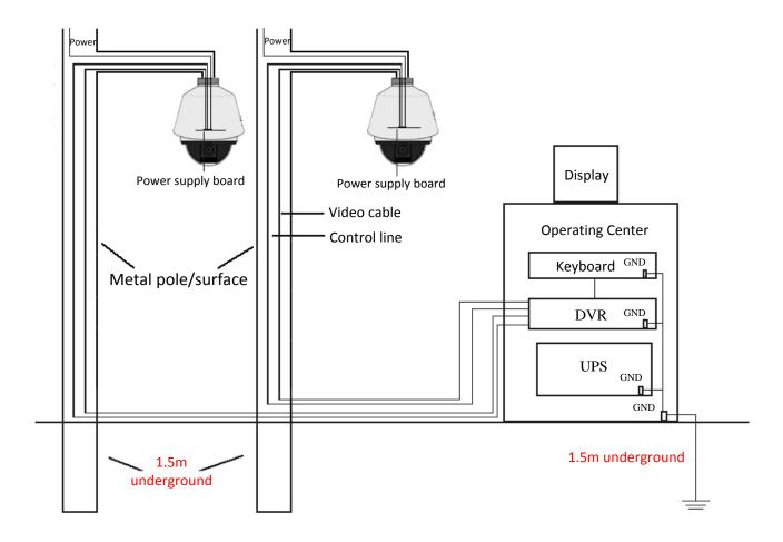
Figure A.3.4 Grounding in Metal Pole Installation
