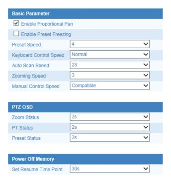
Figure 5-25 Basic PTZ Configuration Interface
