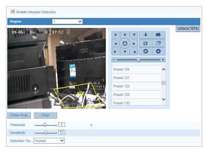
Figure 5-20 Configuring Intrusion Area
