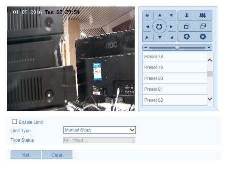
Figure 5-26 Configure the PTZ Limit
