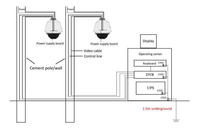
Figure A.3.2 Grounding in Cement Pole/Wall Installation
