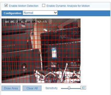
Figure 5-7 Motion Detection Settings-Normal
