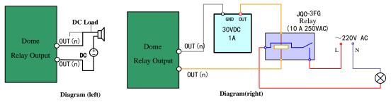
Figure A.10.1 Alarm Out Connections
