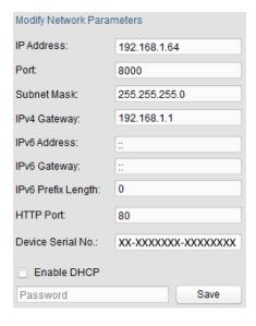
Figure 2-5 Modify the IP Address
