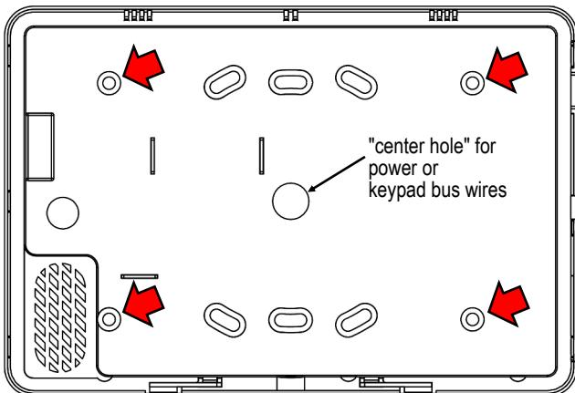
Touchscreen rear case mounting holes for hollow walls (arrows) and the "center hole" for power / keypad bus wires
