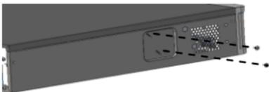
2. Turn the upper mounting plate in the shown direction, then remove the plate.
