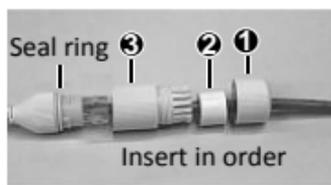
Attach the seal ring to the Ethernet interface. Mount the waterproof components in order. Then insert the cable into the Ethernet interface and screw the waterproof.
