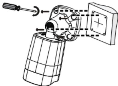
Lead tapping screws through the guide holes in the base and fix them on the wall by using a screwdriver.
