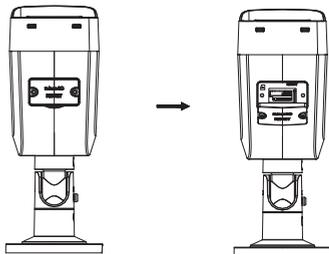
2. Insert the memory card into the memory card slot.
