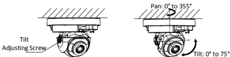
Figure 2-6 2-Axis Adjustment
