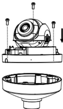
Figure 2-12 Fix the Camera to Cap
