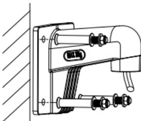
Figure 2-8 Fix the Bracket
