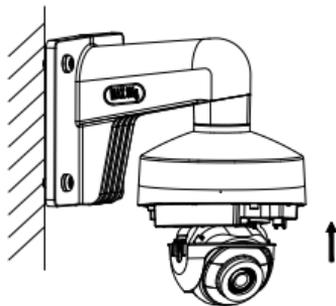
Figure 2-10 Fix the Camera to Wall Mounting Bracket
