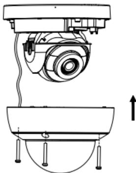
Figure 2-7 Install Bubble
