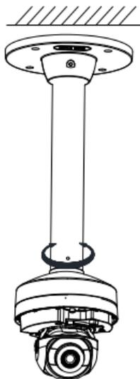
Figure 2-13 Install the Cap
