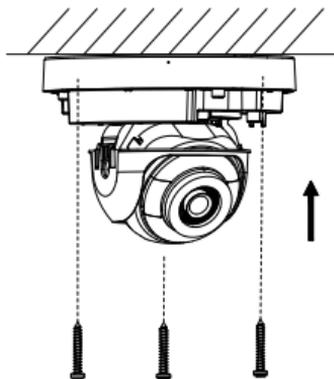
Figure 2-5 Fix the Mounting Base
